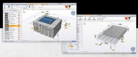
Live calculations change accordingly displaying product optimisation (design life of 50-100 years). Embedment depths are easily adjusted via a drop down menu whilst a series of tabs along the top allow the user to quickly make the amendments to concrete strength, geometry, properties and loads required.
