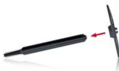
The new insulation support anchor consists of two individual parts, the shank which is installed in the first via an 8mm pilot hole and set by hammer and a separate stress plate...
