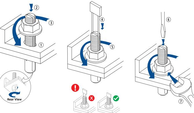
**Rear View** 1. To remove a Blind Bolt release the fixing nut but DO NOT remove it. Push the Blind Bolt further into
