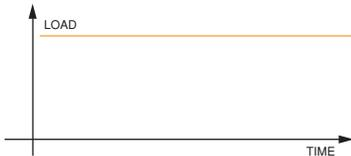
The static or quasi-static loads are dead loads of the element fixed, permanent and variable actions as wind, snow ...
