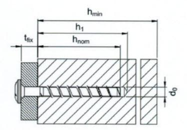
d<sub>0</sub> = nominal drill bit diamter h<sub>nom</sub> = nominal anchorage depth h<sub>1</sub> = depth of the drill hole h<sub>min</sub> = minimum thickness of member
