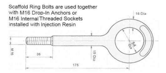
Scaffold Ring Bolts should only be used for scaffold restraint and loaded in tension. They should not be subjected to shear loading.
