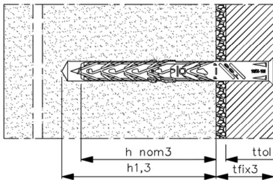
Legend:  $h_{nom,1}$ ,  $h_{nom,2}$ ,  $h_{nom,3}$  = overall plastic anchor embedment depth in the base material
