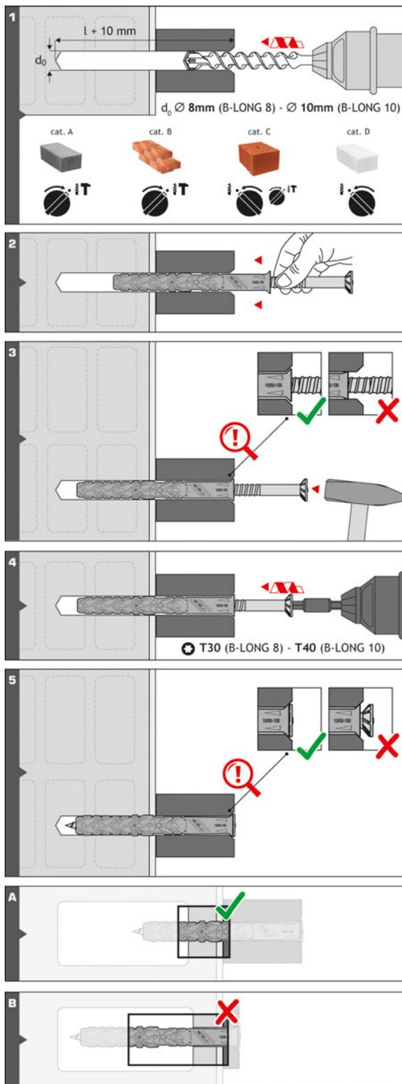
1) Drill the hole considering the drilling method.
