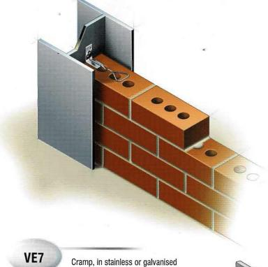
Cramp, in stainless or galvanised steel, for restraining masonry to new or existing structures, and for building in non-structural elements (frames etc.) holed for screwing, bolting or shotfiring, sizes 75mm projection to 150mm, non stock sizes to order.
