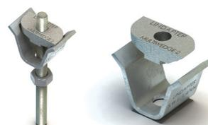
The Alphawedge (AW) is designed to lock quickly and securely into the re-entrant channel of Alphalok or Ribdeck AL decking. The product consists of two parts - a wedge and a plate and has a Safe Working Load of 1kN.
