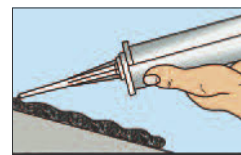
4. Extrude to waste until resin is an even colour
